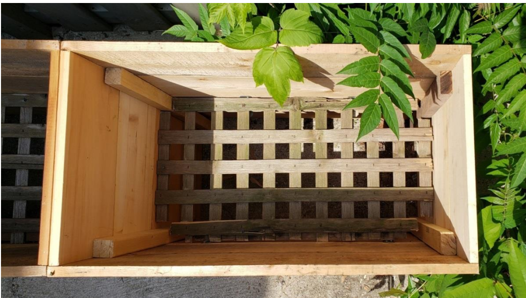
4. View of complete build with corner posts, from above
